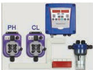
ORP-pH Control system adjusts chlorine dosage by measuring chlorine quantity in water. It measures chlorine level in water then it starts or stops chlorine pumping to water. Depend on the pH value, it provides adjusting dosage quantity. Electrode and electrode cover are present in these models except dosage pump and control panel.
